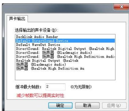
选择声卡输出后，点击开始按钮
